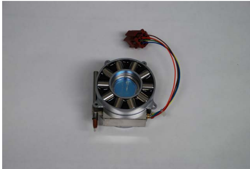
Figure 12 MOF with getter side tube visible on left
