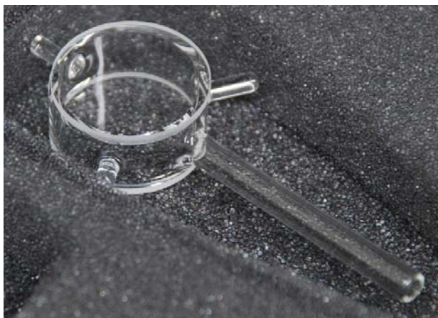
Figure 10 Vapor Cell showing flange posts for tab mounting
